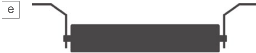
Return roller carries the empty belt on return run.
