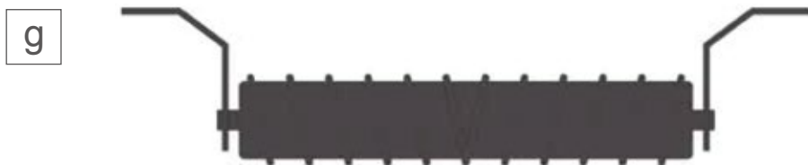
Rubber Disc Return roller used when wet, sticky material tends to cling to the belt. Also used to avoid corrosion .It 's produced in NR or SBR.
